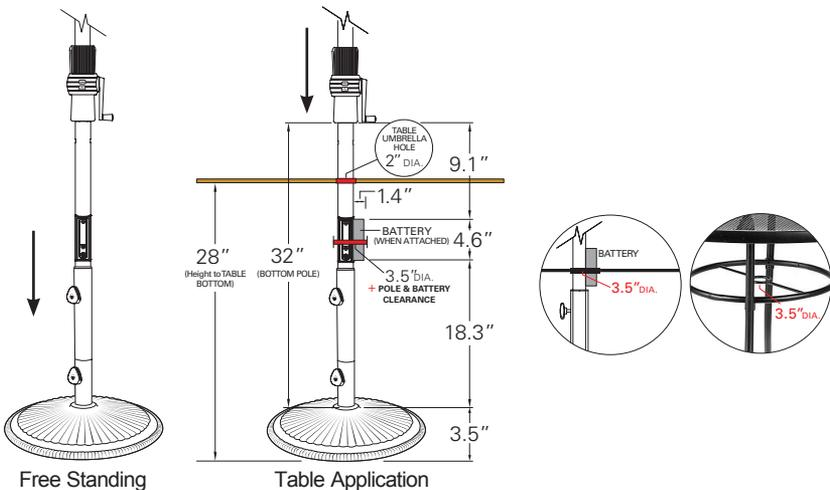
Attach rechargeable battery pack onto bottom pole.
