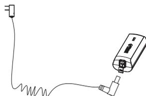
**Battery Status:** Lights on the battery pack will indicate battery charge level. Four lights indicates full charge, while one is low battery. When battery is low, you may charge battery pack while attached to frame, or removed from frame, using power supply included with umbrella.
