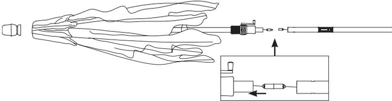
Insert bottom pole onto canopy/mainframe pole. **NOTE:** Make sure battery dock on bottom pole is lined up with ON/OFF switch and USB port on housing. Line up button with hole and snap into place.
